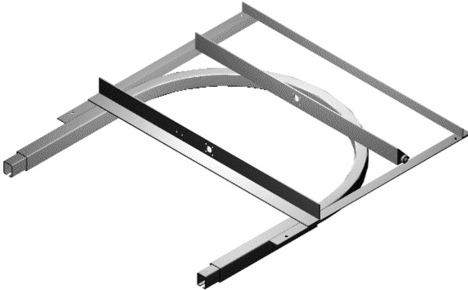
Factory assembled, ready to be hoisted and hung, this frame provides a rigid base and helps make alignment positive. The frame is permanently mounted; only the actuator and conveyor track move. Tensioning is accomplished with your choice of hardware for screw, spring, or air cylinder operation. Available for 2'-0" radius curves (4" maximum track spread).
